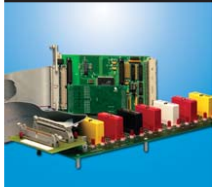
Solid-state relays monitor high/low levels and control the on/off status of various discrete devices.
